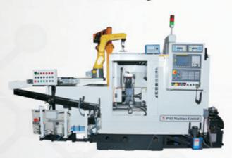
**CNC Cylindrical Grinding**
