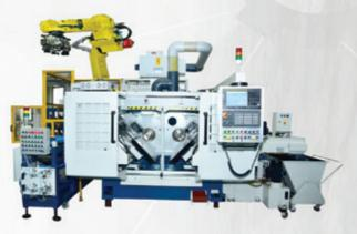
**CNC Twin Spindle Turning**
