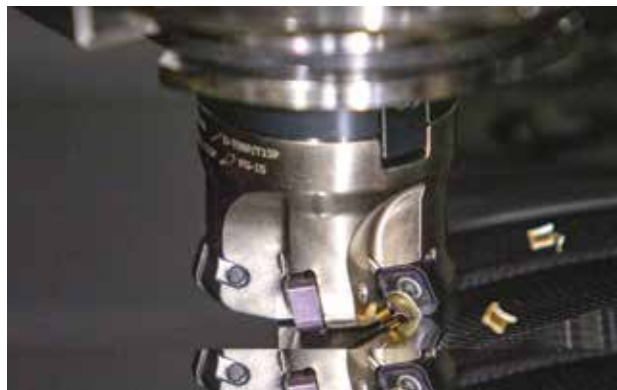
With eight cutting edges, the square-shaped SNGX11 represents an extremely economical solution.
