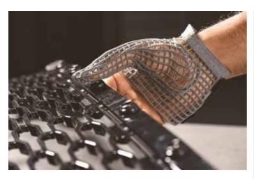
The 3D glove is designed for people working on the production line, for example those required to fit clips or fasteners into the chassis during assembly of Jaguar and Land Rover's luxury vehicles.
