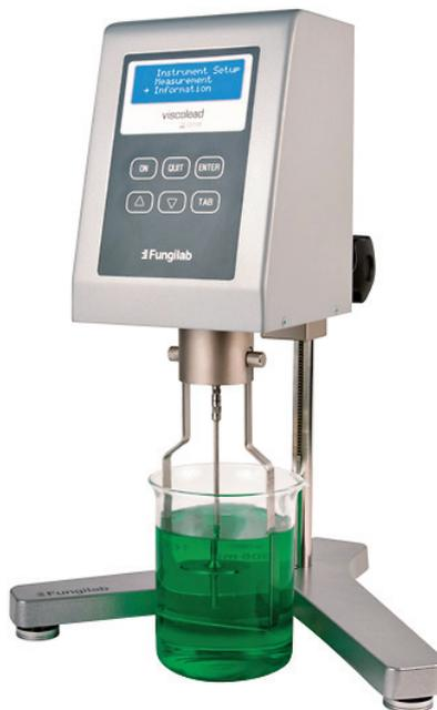
speed, selected spindle, viscosity, percentage torque, shear rate, and shear stress on the 5-line display. Enter the sample density, and the unit calculates and displays kinematic viscosity (cSt) as well.
